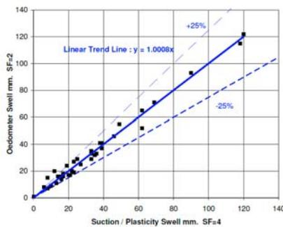
*Comparing strains (y' axis) with suctions (x' axis) reveals a good correlation, improving as the soil becomes increasingly desiccated. A shrinkage factor of 2 has been used for the oedometer, and 4 for suctions.*
