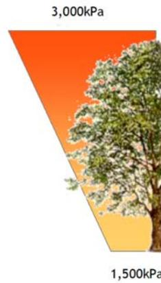
Soil suctions can reach 1,500kPa – this is the point at which suctions exerted by the tree cannot overcome the suctions in the ground. In contrast, atmospheric water potentials can reach very high values depending on the Relative Humidity and temperature, as we saw last month. We have a figure of 3,000kPa but this can easily exceeded, reaching much higher values. Negative pressures within the tree xylem will be at some intermediate value depending on the above.
