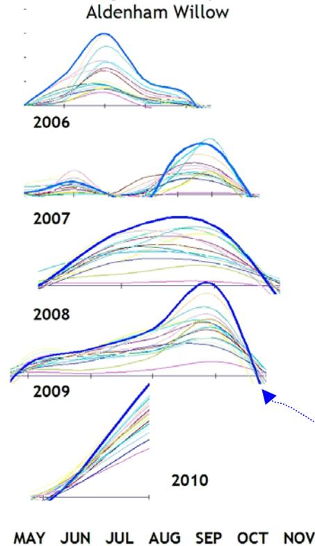
Levelling Station 23 of the Aldenham Willow exhibits more movement than any other. Roots in this location are aggressive pumps, withdrawing moisture resulting in ground movement greater than elsewhere along the two arrays. 2010 reveals that most stations are extracting more water – this graph is based on data gathered on the 8<sup>th</sup> August 2010. Below the plots have been superimposed onto one another to show the increases abstraction in 2010.
