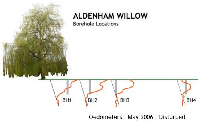
Above are the borehole locations in relation to the tree and one another. Below are the results of investigations undertaken in May 2006 and June 2007. The samples extracted in May 2006 were disturbed. Both disturbed and undisturbed samples were retrieved in June 2007, for comparison purposes.
